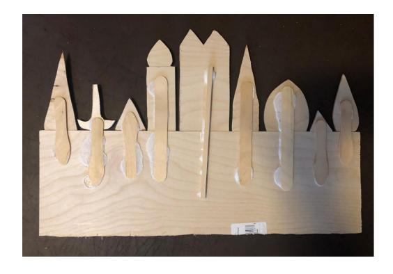
Gorilla Glue is good for attaching pieces of wood or other structural materials together. It's very strong, but be careful not to get it on anything other than the target as it's hard to remove. It also expands quite a bit while drying, so take that into account. Not a lot is needed! Sometimes clamps or weights are helpful for holding pieces together while setting up.
